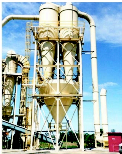
In large cyclone assemblies, service platforms are used to access cyclone maintenance areas and inspection doors.
