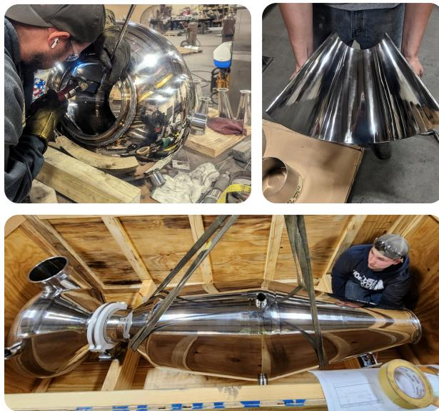
requalification through stringent regulatory pathways. To avoid this, HEC precisely replicated the original geometry, fabricating the system in sections to ensure every contour matched the approved design.
